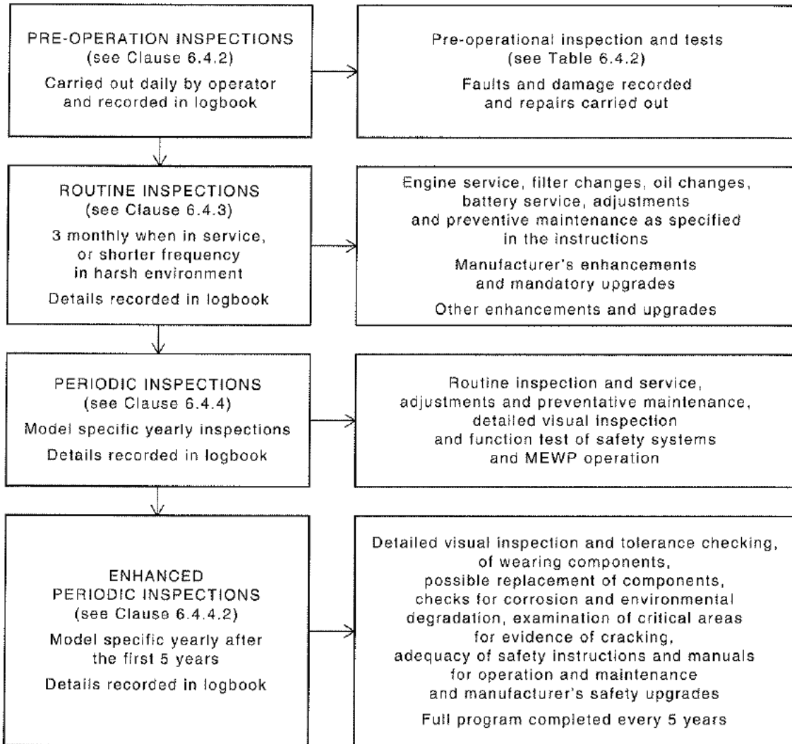
FIGURE D2 MEWPS LESS THAN 5 YEARS OLD AND WHERE MANUFACTURER'S SPECIFICATIONS ARE NOT AVAILABLE, OR ARE DEEMED INAPPROPRIATE OR INADEQUATE BY A COMPETENT PERSON
