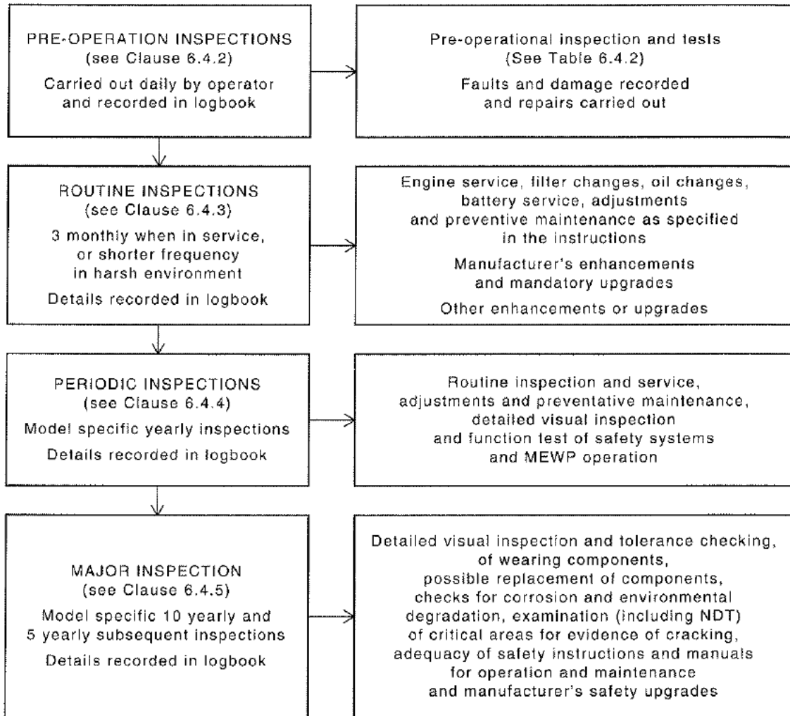
FIGURE D4 MEWPS WHERE MANUFACTURERS SPECIFICATIONS MAY BE INAPPROPRIATE OR INADEQUATE, AND CRITICAL COMPONENTS INSPECTION IS DEFERRED TO THE 10 TH YEAR
